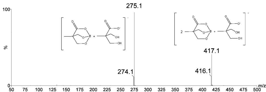
Figure 4. ESI-HRMS spectrum of the formation of diol-monoacid borate with trace of DMPA.
